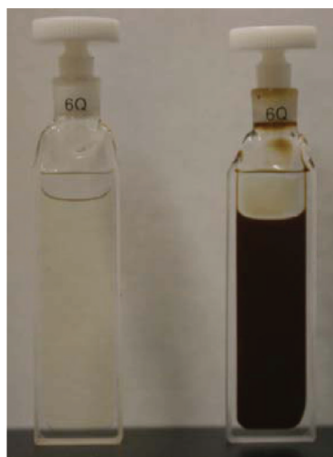
Figure 2. [N_{8881}][Tf_2N] before (left) and after (right) Ag deposition.
